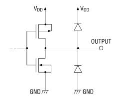
Schematic Diagram of Driver Output Circuit
